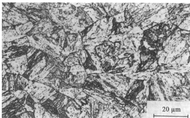
Fig. 1 Microstructure of 1.4914 MANET II steel austenized at 1075 °C/0.5 h, air cooling, tempered at 750 °C for 2 h, and air cooling
